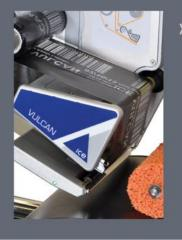
Unique to ICE machines, the clutchless solid state ribbon drive ensures precise and consistent ribbon tension, ribbon save and effortless ribbon changeover, delivering performance and reliability that is unmatched in the industry.
